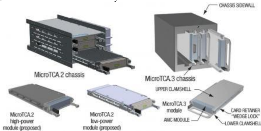
Figure 7: Hardened MicroTCA® module clamshell design allows for the logistical and cost benefits of a two-level maintenance approach.
